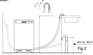
The connection must be made to the hot water line following the same procedures as those for the connection to the cold water line.
